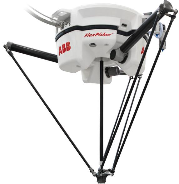
A stainless option for food handling applications is IP69K validated so that it can be washed down with industrial detergents and high pressure hot water. This variant is also designed with smooth and easy to rinse-off surfaces and lubricant free joints that are resistant to most corrosives.
