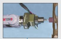
EDGE FINISHING WITH ABRASIVE DRUM
